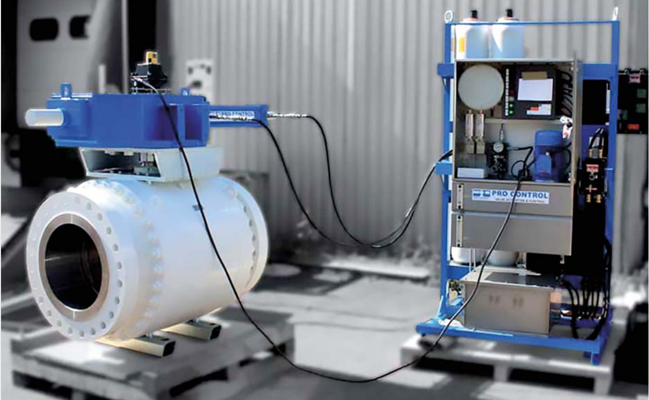
Start-up of HPU (Hydraulic Power Unit) connected with actuated valves
