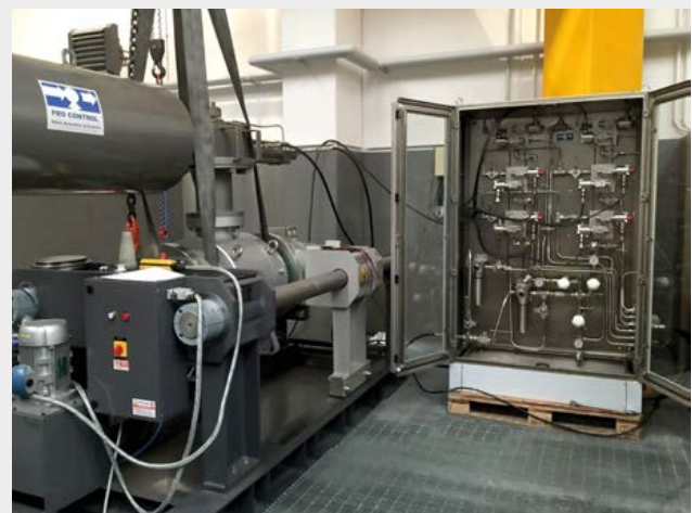
Functional Acceptance Test (FAT) at valve maker factory
